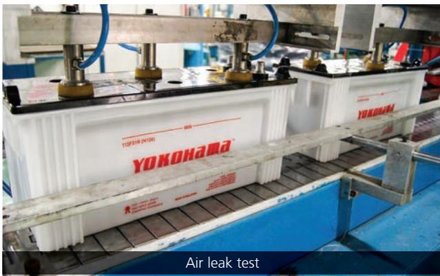
Air leak test
