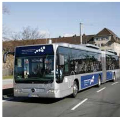
hub motors and the world's largest lithium-ion battery for automotive use. This battery stores the electrical energy from the diesel generator and that recovered by the braking system.
