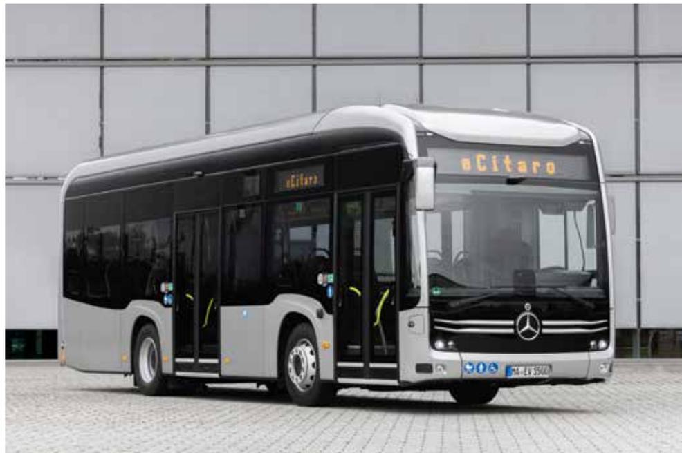
The eCitaro K is available with a minimum of four and a maximum of six battery packs, with a total capacity of up to 588 kWh. In the maximum configuration, the eCitaro K reaches a range of more than 300 kilometres under favourable conditions – over the entire service life of the battery. For even longer routes, intermediate charging using a pantograph is also possible in the eCitaro K.
