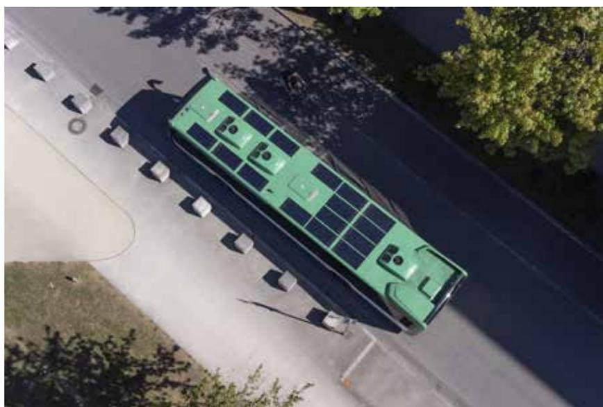
the Mercedes-Benz Citaro and MAN Lion's City, the kit includes lightweight, semi-flexible solar panels that integrate seamlessly onto bus roofs. Each kit can save up to 1 250l diesel per bus per year and up to 3.3t CO2 per bus per year.
